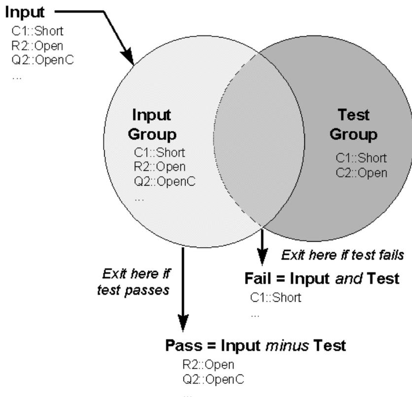
**Figure 2:** Test definition showing the logic used to sequence tests
