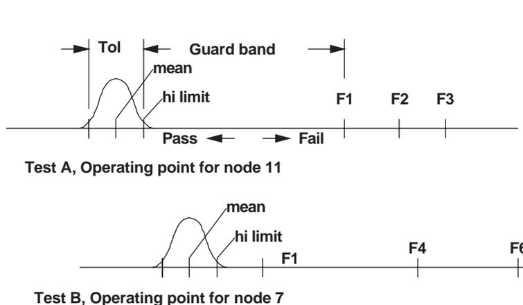
**Figure 4**, Adjusting a test sequence achieves a robust test
