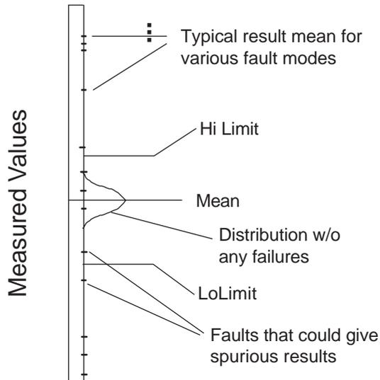
**Figure 1,** Failed parts can result in measurements that are near the measurement limits for normal operation, leading to false conclusions if the test is used for diagnosing those nearby faults
