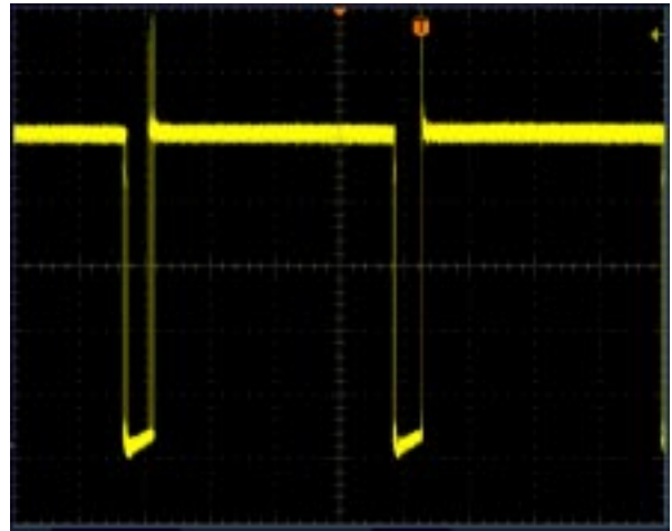
Figure 15. Hardware Oscillograph – VD Voltage Waveform V_{in} = 100 \text{ VAC}/60 \text{ Hz} , R_o = 20 \Omega
