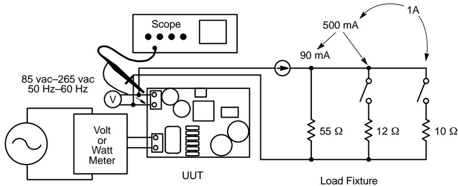
**Figure 1. Power Supply Test Setup**
