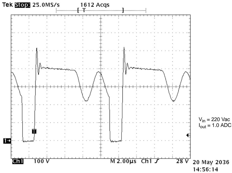
Figure 11. Switching Waveform
