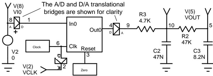
**Figure 7**, This circuit generates the same sine waves shown in Figure 6, however, here a ROM (state machine) is used to driver the filter.
