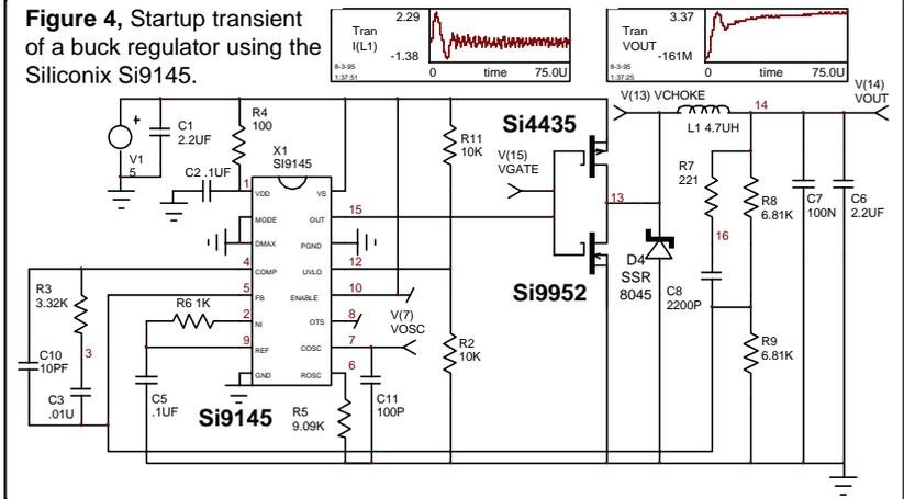
time down. This simulation (.tran 50n 75n 0 10n) takes only 450s on a 486/25. Starting the simulation presented some problems. The .tran UIC keyword is used to initialize the internal logic in the 9145. Unless the VDD capacitors (C1/C2) are initialized with ICs (IC=5V) the VDD pin will start low and ramp to 5V and the switching action will not begin.
