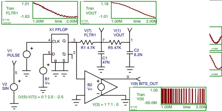
**Figure 6,** Circuit used to generate a sine wave and the 1 bit code representing the sine wave. A portion of the sine wave and bit stream has been cross-probed.
