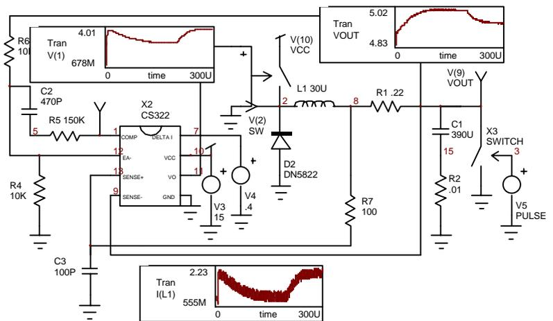
converter using the Cherry CS-322 Hysteretic Current mode controller. The switching frequency is 300kHz.
