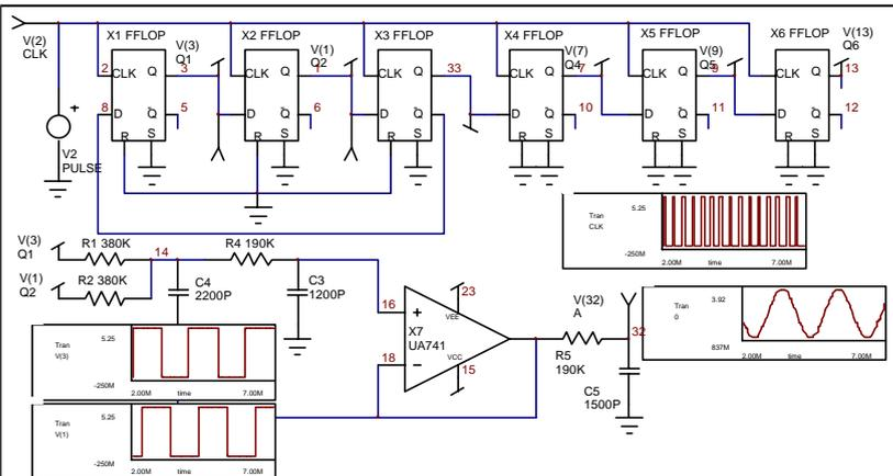
**Figure 8**, Portion of the circuit used to generate a 3 phase sine wave. The taps at the flip-flops are used to drive the active filters. Only one of the 3 phases is shown.
