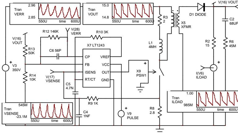
**Figure 1,** Intusoft's New Power Supply Designer's Library allows you to simulate forward converters like this one using the LT1243. See page 2 for more details.
