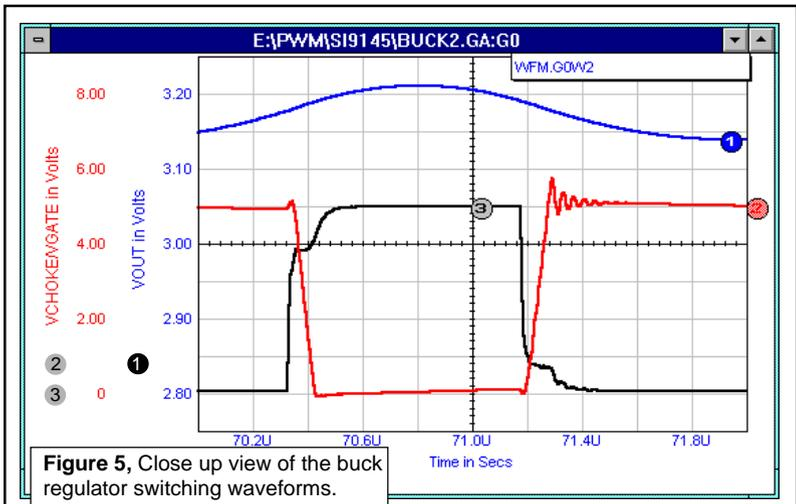
**Figure 5, Close up view of the buck regulator switching waveforms.**
