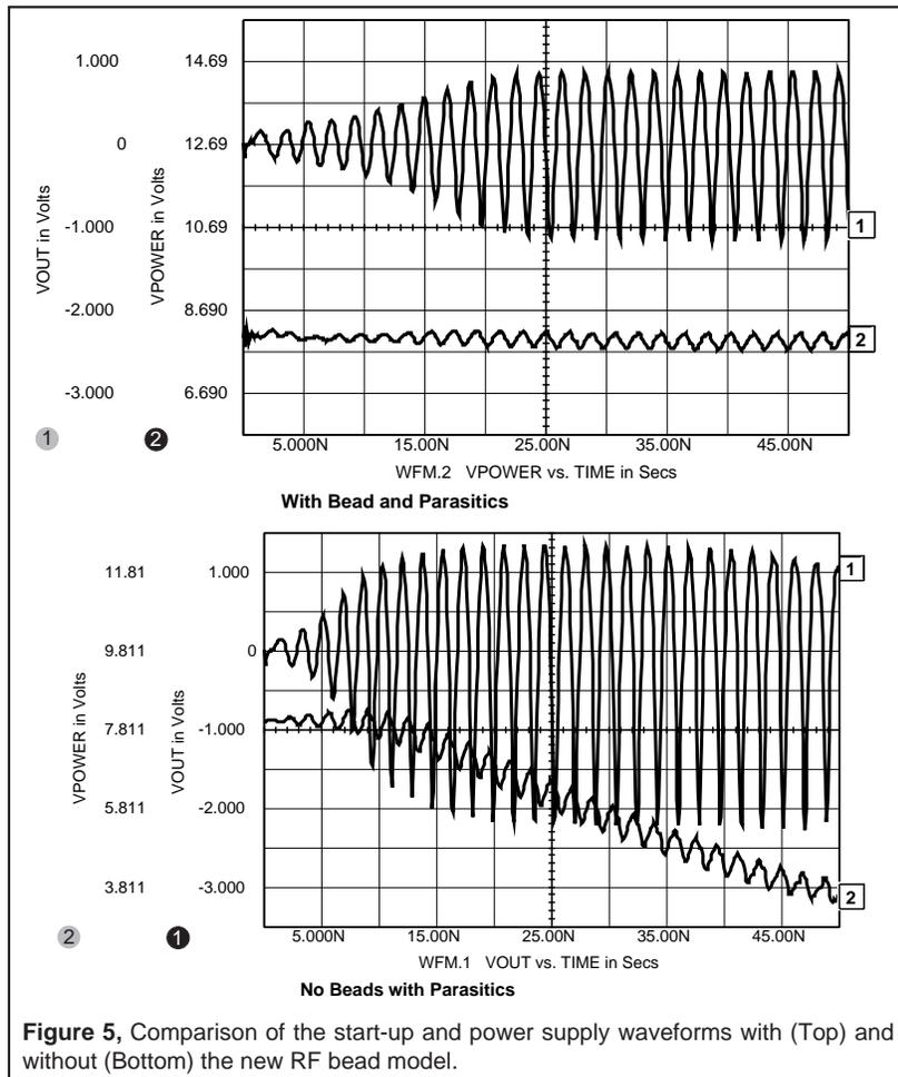
**Figure 5**, Comparison of the start-up and power supply waveforms with (Top) and without (Bottom) the new RF bead model.
