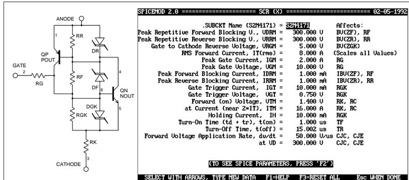
Figure 2, SPICEMOD takes the data sheet parameters shown above and generates an IsSPICE .SUBCKT model (schematic on left) for the SCR. Parameters not available will be estimated by SPICEMOD based on the data that is entered insuring a realistic model.
