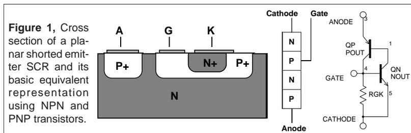
The cathode (emitter) metallization overlaps the gate (base) of the NPN transistor, forming a leakage path to carry leakage currents around the gate until the gate is triggered from an external source. This is shown as RGK in the model.
