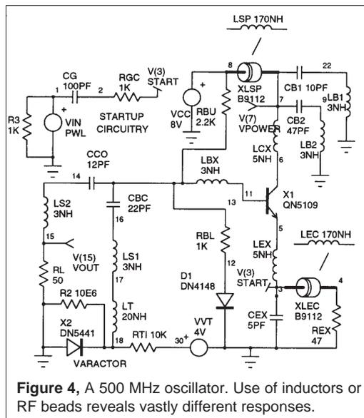
**Figure 4,** A 500 MHz oscillator. Use of inductors or RF beads reveals vastly different responses.
