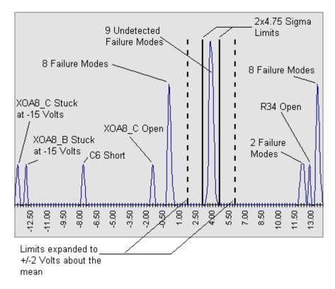
Figure 3 - Failure information shows limits can be expanded without affecting test results.
