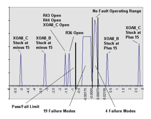
Figure 2 - Node 138 Voltages For Failure Modes and No Failure
