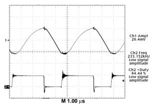
Trace 1– Regulator Output Voltage (10 mV/div.)
