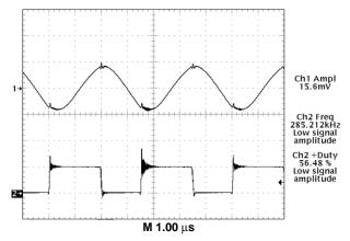
Trace 1- Regulator Output Voltage (10 mV/div.)
