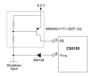
Figure 16. Implementing Shutdown with the CS5155
