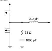
Figure 20. Filter Components
