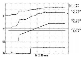
Trace 3 – 12 V Input ( $V_{CC1}$ ) and ( $V_{CC2}$ ) (10 V/div.)
