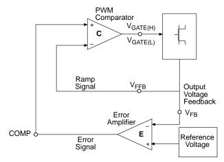
Figure 3. V<sup>2</sup> Control Diagram
