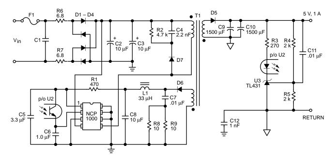
Figure 2. Schematic Diagram
