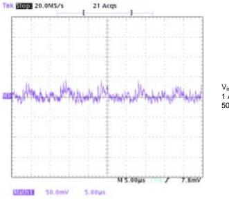
V<sub>in</sub> = 115 V<sub>rms</sub> 1 Amp Load 50 mV/div, 5 µs/div
