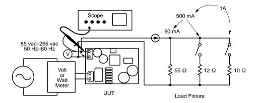
Figure 1. Power Supply Test Setup
