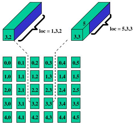
The first dimension of the dim parameter, 20, establishes the time vector size. This is the depth of each element shown in the figure. The following two dimensions provide the number of rows and columns in the array node matrix. In all, we will have 30 time vectors each having a size of 20.
