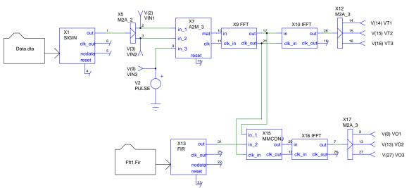
Recall that the output of the previous example was the impulse response of the RC circuit. The data collected represent the impulse coefficients for the filter. These coefficients are used in a frequency domain multiplication to filter the signals collected by the Data.Cir example.
