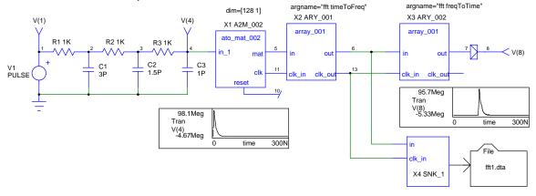
In this example we find two new Array elements, X2 and X3, performing an FFT and an IFFT respectively. The remaining elements have been discussed in other examples.
