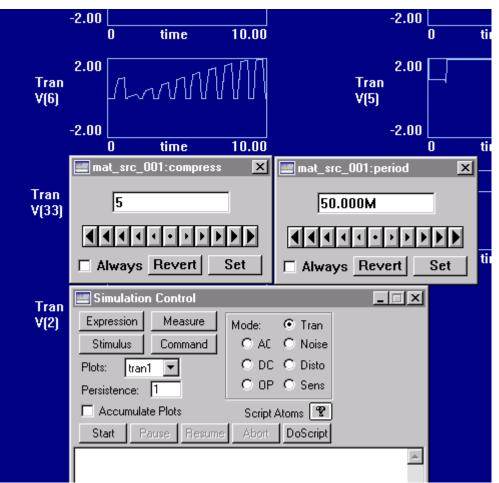
There are several ways to get a graphical view of an array node. In the examples all of them. In HelloC.cir a wavelet compressed node is to be viewed. This requires special processing. Render is a 32 bit InProcess Server that connects to OLE compliant container application and allows array data to be viewed in real time.
