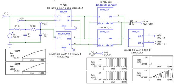
This circuit will look very similar to the previous example. The only difference is the resolution that takes place at node 4. To resolve the parallel connection the two arrays are summed to create the output that is passed to the next array model.
