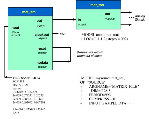
The server for mat\_src is source.dll. The server is accessed by setting the op model parameter to source. (op="source") At this time this is the only server available for the mat\_src model.
