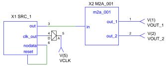
The two main components of this circuit, X1 SRC\_1 and X2 M2A\_001, have been discussed in previous examples. The new feature we are demonstrating is controlled by the Source Array model found in SRC\_1. The model statement is shown below.
