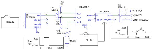
The element of interest here is the convolution element, X7. This model eliminates the need for the FFT, IFFT and MMCONJ blocks of the previous example. The model statement for the array model is shown below.
