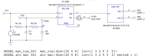
The Array-to-Matrix bridge, X1, uses a 20x5x6 matrix as the array node. This matrix is established by the dim model parameter shown in the ato\_mat model. The matrix is shown in the following figure.
