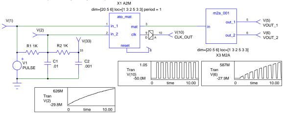
Each new period will generate new data that is placed in the array matrix established for the circuit. There are no new array matrices created during the simulation. Each set of data replaces the previous.
