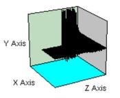
Each of the traces in the 3D graph shown above keeps the largest values in wavelet space, nulling out the remaining values. This would give a constant bandwidth solution, even when no sound is present; clearly a better solution is to set an absolute threshold in order to eliminate silent periods. You may wish to make your own compression/decompression algorithm and test it using SALT!
