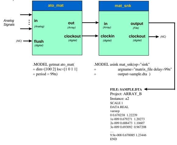
The server for mat\_snk is sink.dll. The server is accessed by setting the op model parameter to sink. (op="source") At this time this is the only server available for the mat\_snk model.
