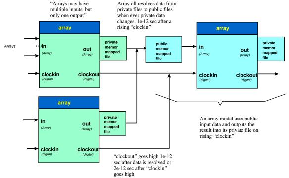
When 2 array outputs are connected together, a process called resolution takes place. Resolution can be either by summation, replacement, or a combination of the two. The resolution method for the baseline array models is hard coded into the models, and is the basis for stripping out certain array channels for analog processing and their later re-insertion into the array data structure.
