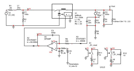
Figure 4, Example of peak current control PWM using external STATESET shown in A2 and A3.
