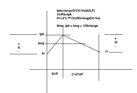
Figure 2, Basic waveform describing peak current control
