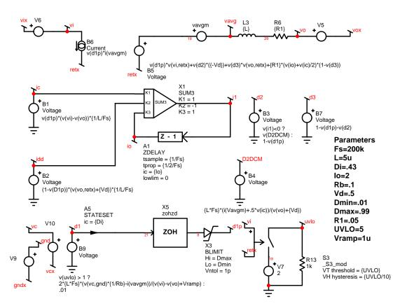
Figure 3, An IsSpice4 average PWM model for peak current control.
